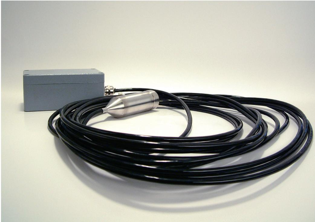
Electronic transmitter with submersible measuring probe in stainless steel for level measurement in vessels where pressure connection in the bottom is not possible or desirable. For example pump pits, reservoirs or plastic tanks.
