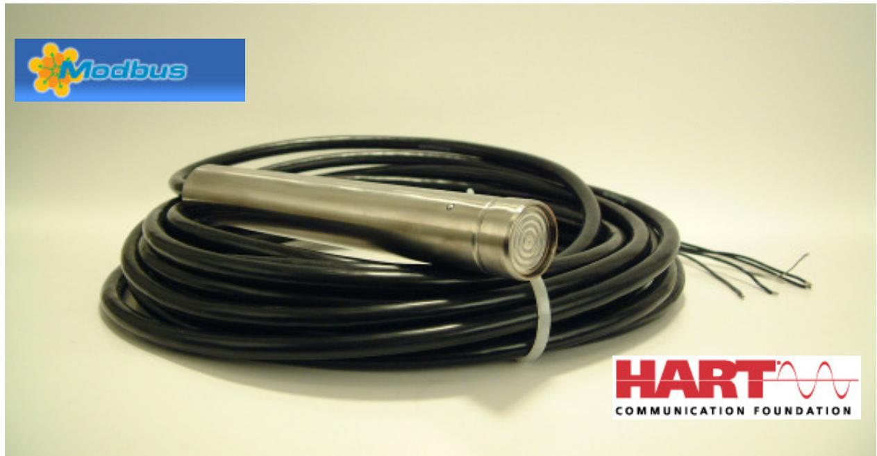
Level transmitter with submersible probe in stainless steel for level measurement in vessels where pressure connection at the bottom of the vessel is not possible or desirable. For example pump pits, reservoirs or plastic tanks.
