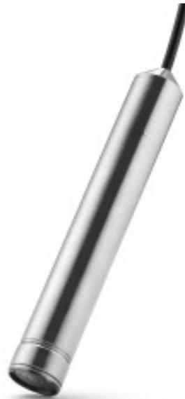
Level transmitter with submersible probe in stainless steel for level measurement in vessels where pressure connection in the bottom of the vessel is not possible or desirable. For example pump pits, reservoirs or plastic tanks.
