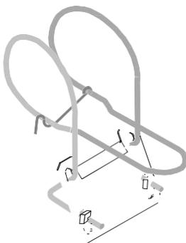
Mount the Flexible Mounting Bracket on handrail diameter of 1 1/4" – 2" (32-50 mm) Ø or square 1 1/8" – 1 5/8" (28-42 mm). The bent lip on the mounting plate shall be on top and faced toward the liquid or tank. Adjust the Mounting Bracket to the correct angle and tighten the SS nuts. The bracket shall be fixed to the rail, and it shall not be able to move it.
